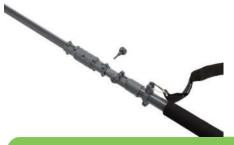
IMPORTANT! If the two sections are not connected correctly, there will be intermittent or no power. If this is so, check the connection is fully engaged.
